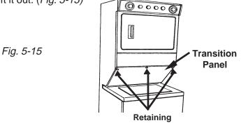
2. Release the two washer top retaining clips and slide the washer top forward off the unit. *(Fig. 5-16)*
