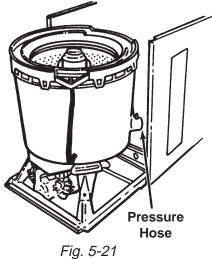
5.Lift and pull the washer assembly forward out of the cabinet. From this position it is possible to service all the washer components, which are similar to those used in other Whirlpool direct drive washers.
