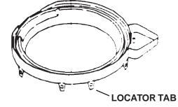
3. The Surgilator Agitator is removed by first pulling off the agitator cap and inner cap. Then unscrew the 7/16" bolt found under the cap and pull straight up on the two-piece agitator assembly. The clutch and clutch dogs that provide the Surgilator action are found in the upper portion of the agitator assembly. (*Fig. 3-15*)
