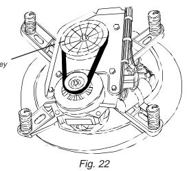
6. The splutch housing is held to the motor plate by four tabs. Work each tab loose by pressing in while pulling out on the housing until it is free.
