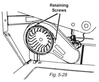
**NOTE:** The Blower is reverse threaded and is removed by turning it clockwise.
