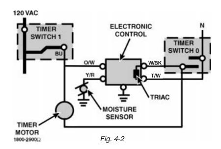
The electronic control looks at the input from the moisture sensor to see if the clothes are wet or dry. The moisture sensor will show continuity (short) if the clothes are wet and show **NO** continuity (open) if the clothes are dry.
