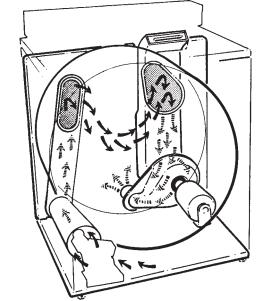
Air system is similar in gas and electric dryers. Gas Dryer shown.
