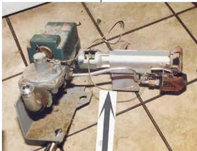
The most common problem is caused by the pilot light combustion byproducts. The flame leaves behind small amounts of ash and the capillary is not heated properly in the flame. The same *Uncle Harry's* tip applies.
