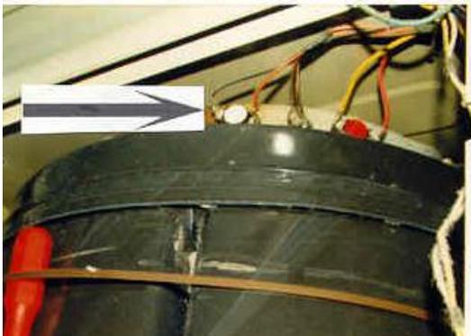
The elements come as a pair and need to be re-strung through all the insulators that are mounted to the back of the dryer. It takes some time to re-string the element properly. Care must be taken not to stretch the element too much when you're re-threading. The element should be threaded so that it has a slight tension on it after you're finished and it looks neat and tidy and is not close to any metal.
