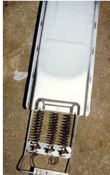
On Whirlpool the heating element slides into a long sheet metal box which is clamped onto the rear of the dryer. The bracket that holds the heater box is held in by one screw. The small bracket squeezes the heating element chamber up against the back of the rear basket frame. It is accessible in two ways.
