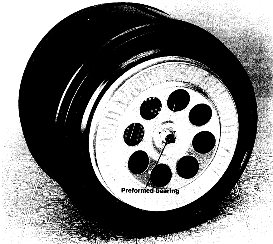
Drum bearing located on rear drum shaft
