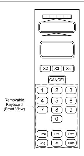
Scanner Panel with Removable Keyboard Installed
