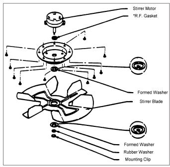
**NOTE:** Formed washers were used on early production only. Formed washers are not used with replacement stirrer blades.
