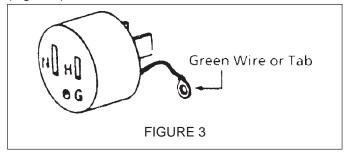
**NOTE:** The green wire or tab should be connected to a proper ground by a qualified electrician.
