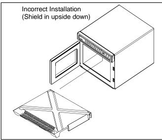
NOTE: If splatter shield is installed upside down, shield will interfere with antenna movement.
