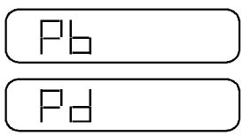
• "Pb" or "Pd"—Indicates programming mode and current menu. See "Programming" section of manual for programming procedure.
