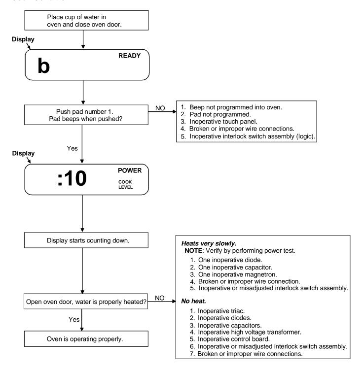
NOTE: Shut down after cook cycle - door closed - 25 seconds. Shut down, door open - approximately 5 minutes.
