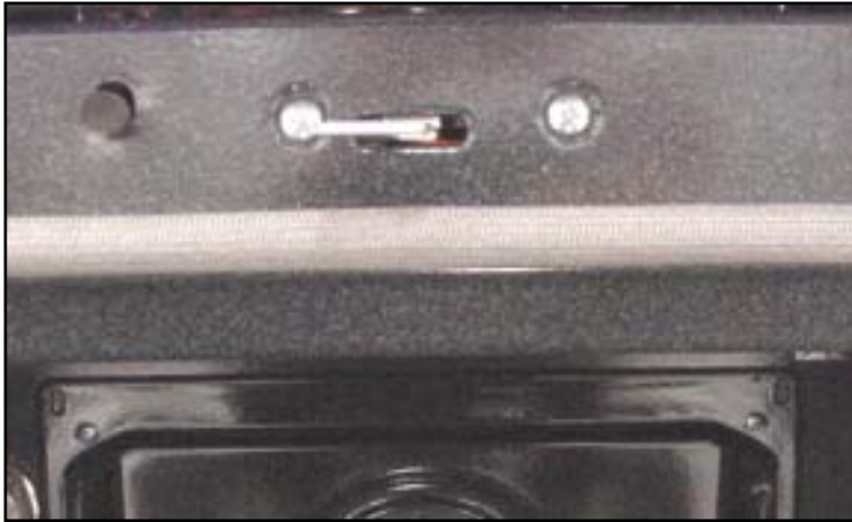
Remove 2 screws from front frame
