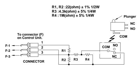
**Sensor Dummy Resistor Circuit**
