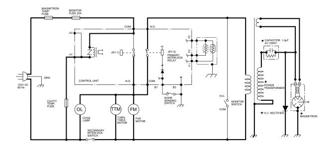
Figure O-2. Oven Schematic-Cooking Condition
