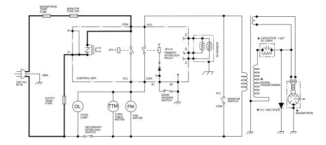
Figure O-1. Oven Schematic-Off Condition
