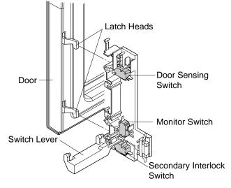
Figure C-3. Latch Switch Adjustments
