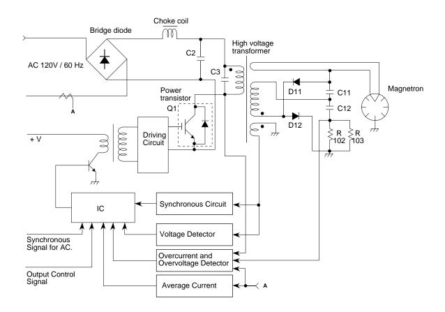
Figure A-1. Basic Circuit
