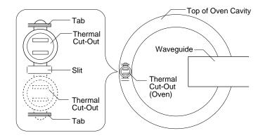
5. Remove one (1) screw holding the thermal cut-out to the
