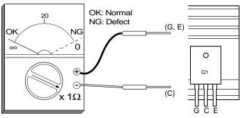
Figure B-2. Check for Power Transistor Q1
