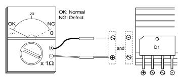
Figure B-4. Check for bridge diode D1.
