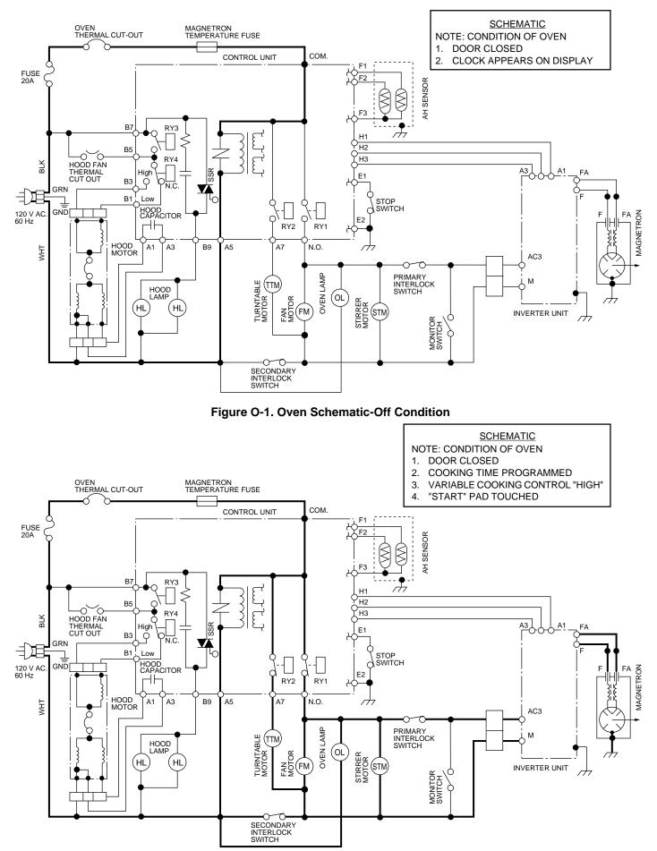
Figure O-2. Oven Schematic-Cooking Condition
