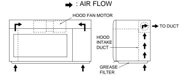
3. RE-CIRCULATION (INSIDE VENTING) The air handing is the same as VERTICAL VENTING except that the final air discharge is directed horizontally through the upper front of the oven into the kitchen. In this case, the accessory charcoal filter RK-230 must be provided to filter the air before it leaves the oven.
