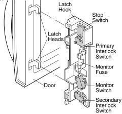
Figure D-1. Door Open Mechanism
