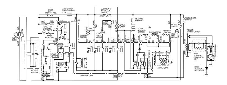
Figure O-2. Oven Schematic - Microwave Cooking Condition
