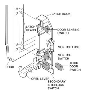
Figure C-1. Latch Switch Adjustments
