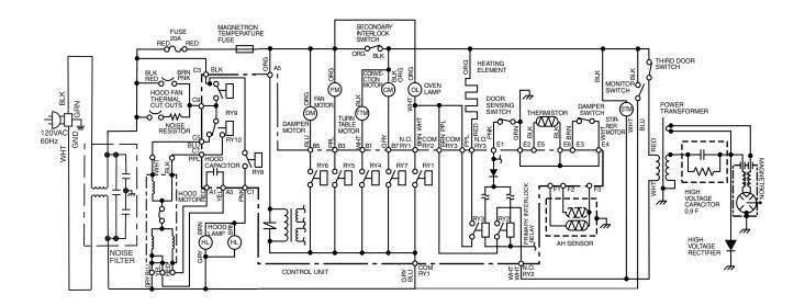
Figure O-1. Oven Schematic - Off Condition
