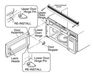
Figure C-2. Door Replacement and adjustment
