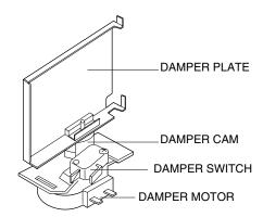
Figure D-2. Damper Mechanism
