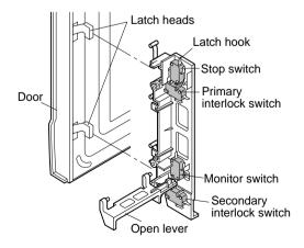
Figure C-1. Latch Switch Adjustments
