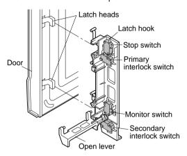
Figure D-1. Door Open Mechanism
