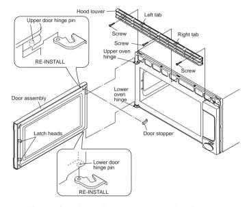
Figure C-2. Door Replacement and adjustment
