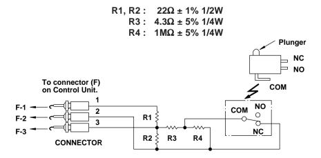
**Sensor Dummy Resistor Circuit**
