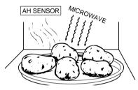
3. Sensor detects moisture and humidity and calculates cooking time and variable power.
