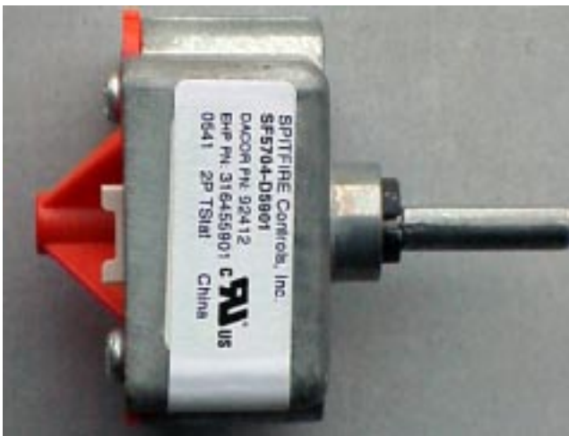
temperature selector mounted to the console,
