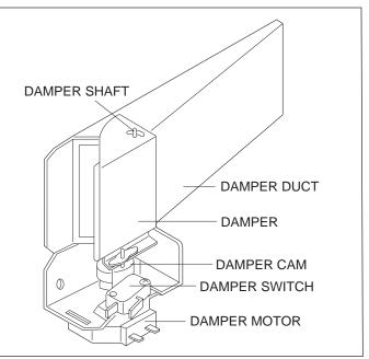
Figure 2-8. Damper Assembly
