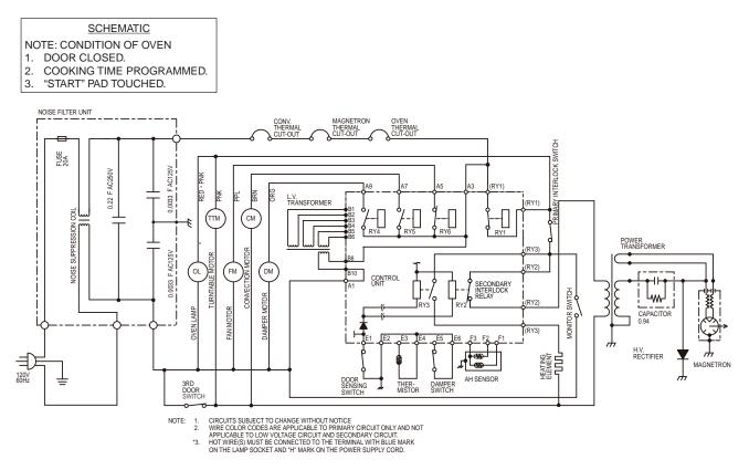
Figure 2-2. Oven ON (Cooking) Condition
