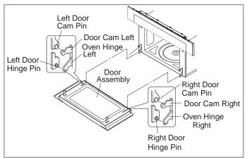
Figure 4-7. Door Assembly Components
