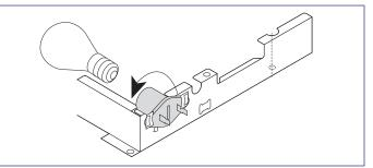
Figure 4-1. Oven Lamp Socket
