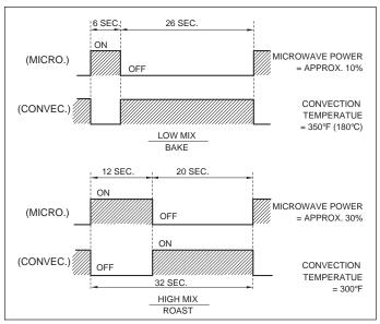
Figure 2-3. Automatic Mix Cooking Cycle
