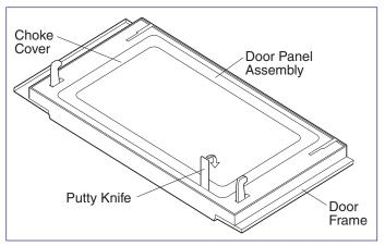
Figure 4-8. Door Disassembly
