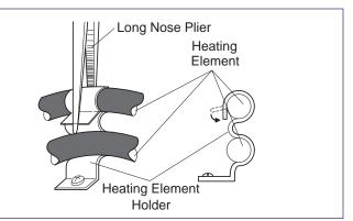
Figure 4-4. Heating Element Removal
