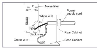
Figure 4-3. Power Cord Connections
