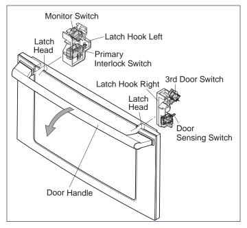
Figure 4-5. Door Switch Components
