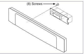
Figure 4-9. Control Panel and CPU
