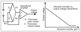
Figure 2-7. Humidity Sensor Operation
