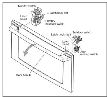
Figure 2-5 . Door Sensing Switch, Monitor Switch, Third Door Switch And Primary Interlock Switch
