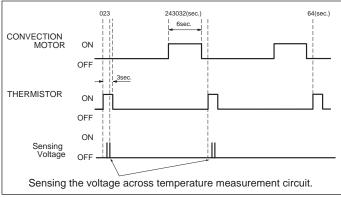
Figure 2-4. Fire Sensing Feature
