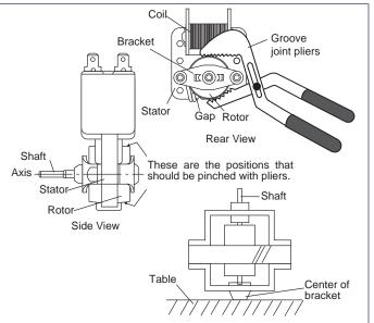
Figure 4-2. Fan Motor Components
