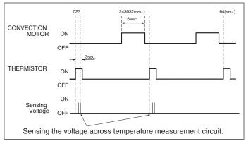
Figure 2-4. Fire Sensing
