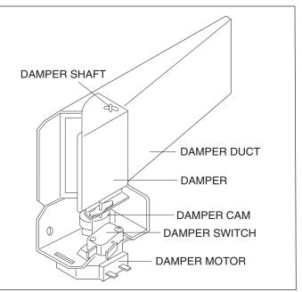
Figure 2-7. Damper Assembly
