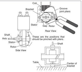
Figure 4-2. Fan Motor Components
