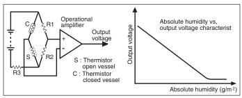
Figure 2-7. Humidity Sensor Operation
