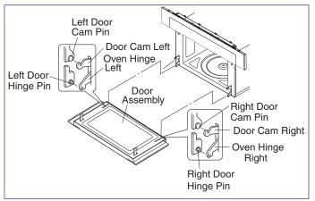
Figure 4-7. Door Assembly Components
