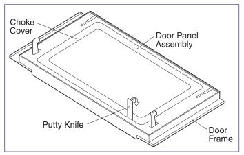
Figure 4-8. Door Disassembly
