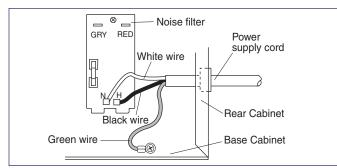
Figure 4-3. Power Cord Connections
