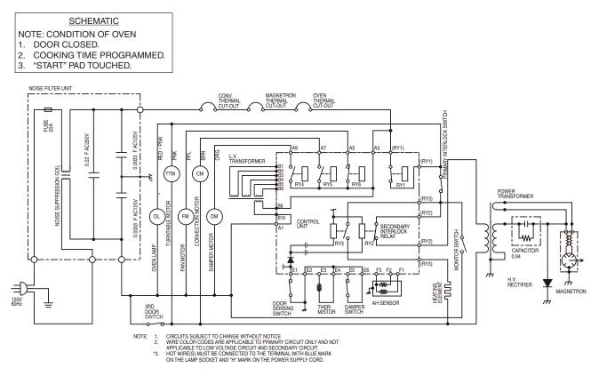
Figure 2-2. Oven ON (Cooking) Condition
