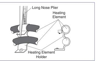
Figure 4-4. Heating Element Removal
