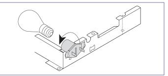
Figure 4-1. Oven Lamp Socket
