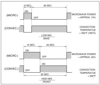
Figure 2-3. Automatic Mix Cooking Cycle
