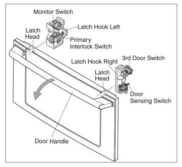
Figure 4-5. Door Switch Components
