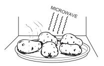
3. Sensor detects moisture and humidity and calculates cooking time and variable power.
