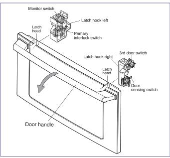
Figure 4-4. Door Switch Components
