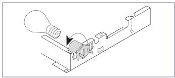
Figure 4-1. Oven Lamp Socket
