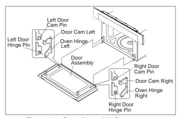
Figure 4-6. Door Assembly Components
