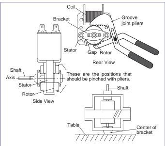
Figure 4-2. Fan Motor Components
