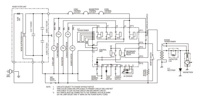
Figure 2-2. Oven ON (Cooking) Condition
