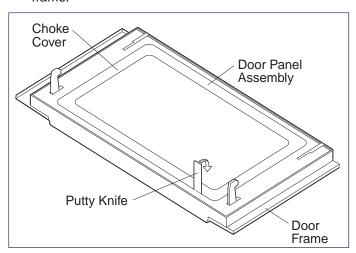
Figure 4-7. Door Disassembly
