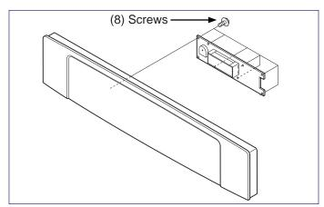
Figure 4-8. Control Panel and CPU
