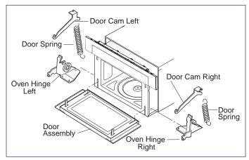
Figure 4-5. Door Replacement and Adjustment
