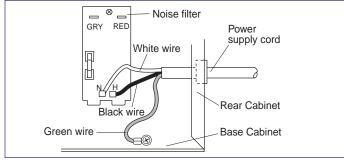
Figure 4-3. Power Cord Connections
