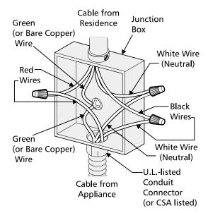
Figure 6 4-Wire Electrical System (example: Junction Box)
