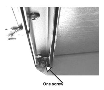
9. Remove one screw holding the lower brace to the side panel and lift the panel off.
