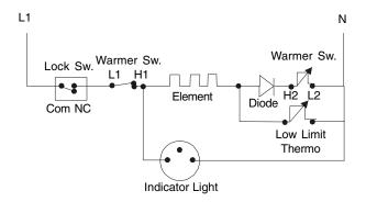
Preheat or the first cycle is controlled by the low limit thermostat which is set to open at about 150° F and reclose at about 140° F. The low limit thermostat is connected electrically in parallel with the diode and
