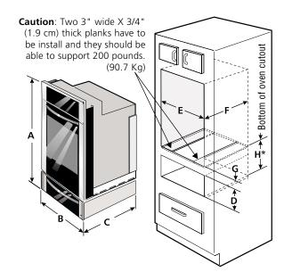
$H^* = 10 \text{ } 1/8^{\circ} \text{ } (25.7 \text{ } \text{cm}) \text{ Min. is a Critical dimension and has to be respected.}$
