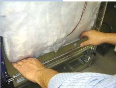
**4.12** Push the insulation back into its original emplacement making sure that it's properly tucked in behind the lower panels.
