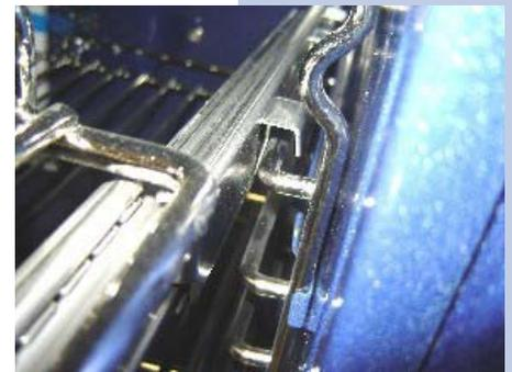
**5.41** To remove the ladder rack from the oven liner, push the ladder racks up in order to free them from their holders.
