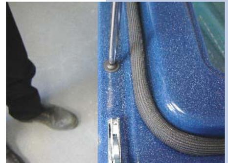
**13.9** Remove the 9 screws that hold the inner door baffle.
