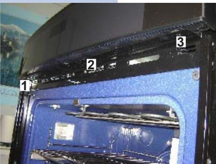
**1.4** Remove the 3 screws from under the control panel.
