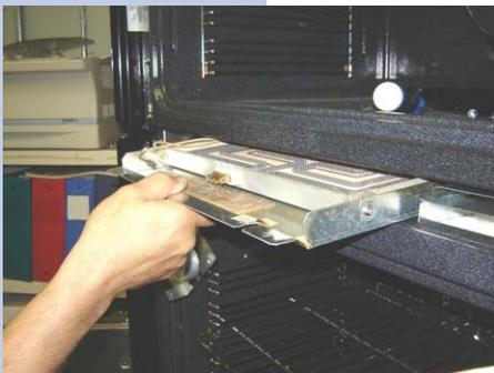
**11.5** Remove the hidden bake element from between the upper and lower oven frames.
