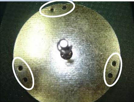
**9.9** Properly align the mounting holes from the mounting plate and the convection motor. From the front side of the convection motor...
