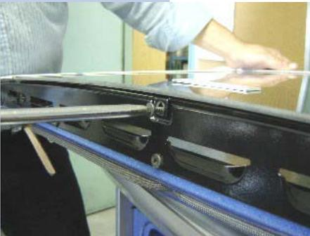
**13.3** Remove the center screw of the lower trim; the one closest from the oven door glass.
