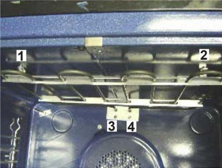
**8.1** Remove the 4 screws from the broil element
