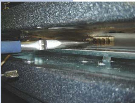
**11.4** Using a pair of long nose pliers, remove the 2 hidden bake wires.
