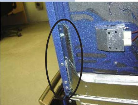
**4.11** Locate hinge receptacle from the side and remove from the back of the front frame.
