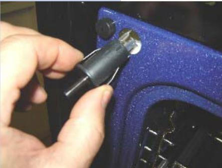
2.3 Gently pull on the automated door light switch and remove from the unit.
