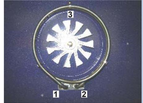
**9.3** Pull the convection element out and unplug the two orange wires.
