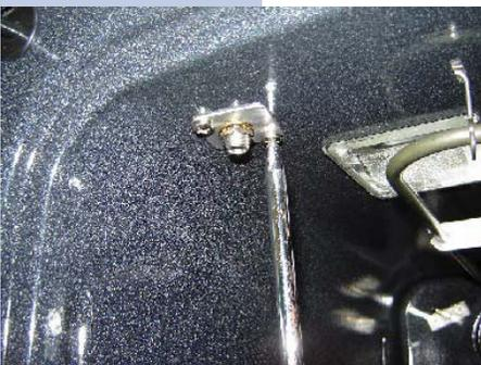
**6.1** Unscrew the two screws which hold the meat probe receptacle to the upper portion of the oven liner.
