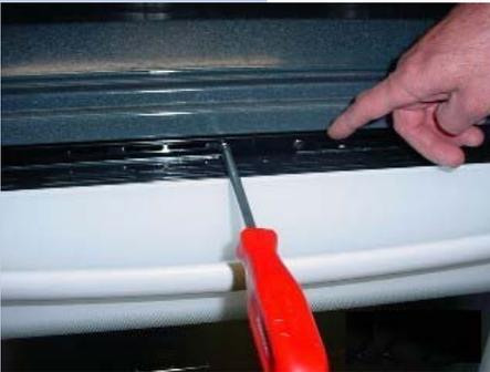
**3.13** Remove the two screws which holds the door lock assembly to the center trim.
