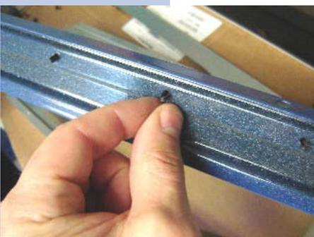
**13.16** Apply pressure (squeeze) on the spring clip of the oven door gasket in order to remove it.
