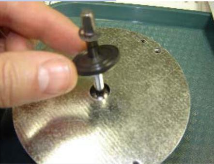
**9.8** Remove the rubber washer from the convection shaft.
