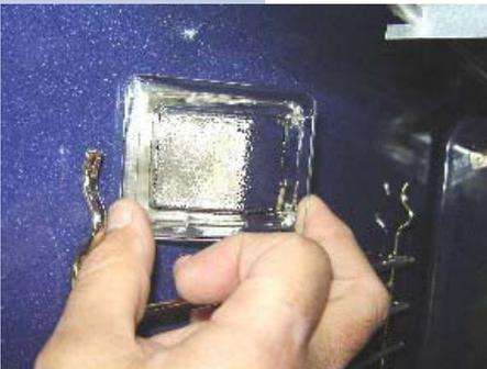
**5.5** Gently pull on the light cover in order to have access to the halogen lamp.
