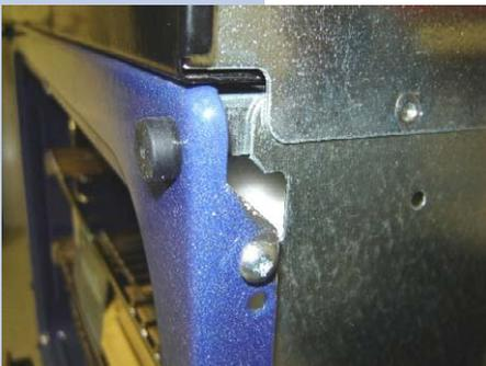
**4.13** Upon replacing the side panel, make sure that it will be inserted between the frame and the upper side panel as shown.
