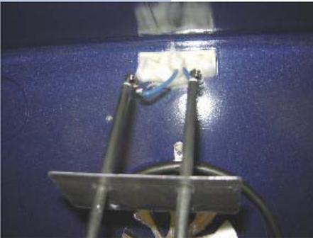
**8.2** Pull the broil element out and unplug the two blue wires.
