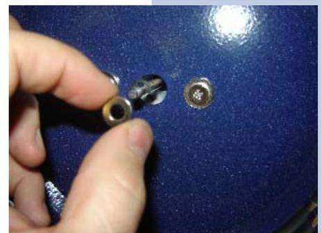
**9.7** Remove the 4 screws from the convection motor and remove from the unit.
