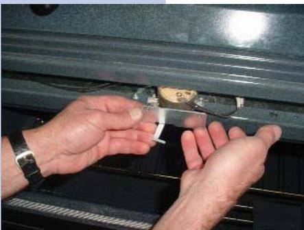
**3.15** Remove the door lock assembly from between the two oven liners and unplug all wires.
