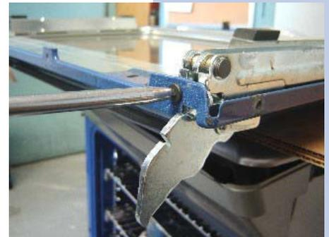
**13.8** Turn the oven door upside down and remove the screw that holds the oven door hinge to the inner door liner.
