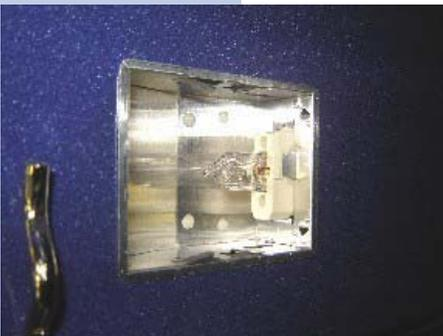
**5.6** Gently pull on the halogen lamp in order to remove it from its socket.
