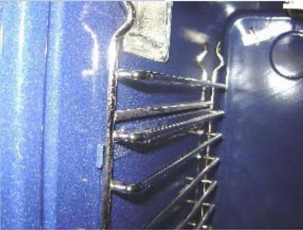
**5.42** View of the ladder rack out and ready to be removed from its holder.
