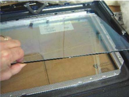
**13.12** Remove the 2<sup>nd</sup> inner glass from the glass pack assembly.
