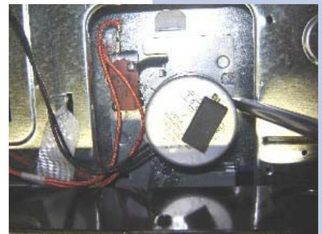
**3.6** Remove the door lock assembly; unplug all wires and quick connector in order to replace the door lock assembly....
