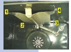
**13.1** Remove the 4 screws which hold the broil burner assembly in place.
