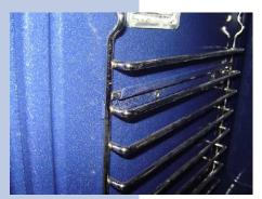
**7.41** To remove the ladder rack from the oven liner, push the ladder racks up in order to free them from their holders.
