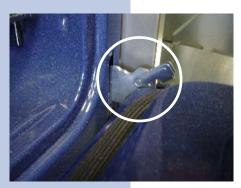
**1.2** After locating the hinge lock lever, pull it to the lock position as shown.
