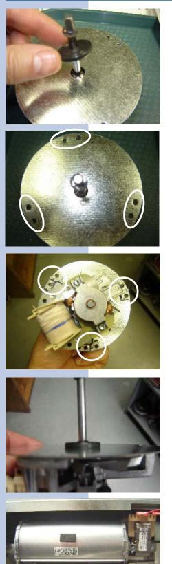
11.8 Remove the rubber washer from the convection shaft.
