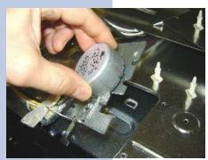
**4.7** Remove the door lock assembly; unplug all wires and quick connector in order to replace the door lock assembly....
