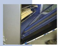
**1.3** Pull the oven door up at roughly 45° as shown; this will lock the oven door hinges, and pull the oven door out of its hinge receptacles and away from the unit.
