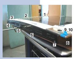
**20.4** Remove the 10 screws that hold the front decorative glass assembly; 4 at the top and 3 on each of the left and right hand side.
