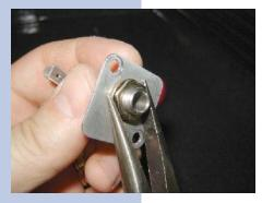
**9.3** Unscrew the nut which hold the meat probe receptacle to its mounting panel.
