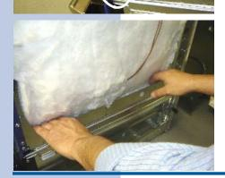
**8.12** Push the insulation back into its original emplacement making sure that it's properly tucked in behind the lower panels.
