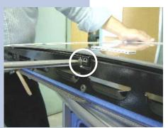
**20.3** Remove the center screw of the lower trim; the one closest from the oven door glass.
