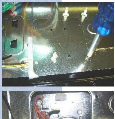
**4.5** Remove the 1 screw that holds the service panel in place.
