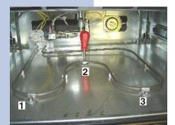
**18.5** After having removed the A & B screws, (16.4) using a small screwdriver, remove the 3 screws that hold the warmer drawer element.
