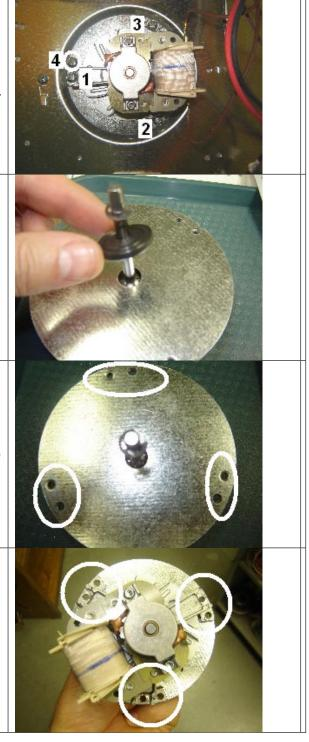
**11.10** Make sure that the rubber washer is properly installed; laying flat on the convection motor mounting plate.
