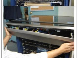
**1.8** Gently pull the control panel down and off of the unit.
