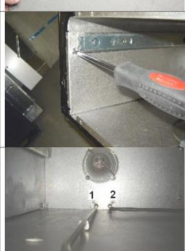
**13.4** Remove the 2 screws from the mini oven bake element
