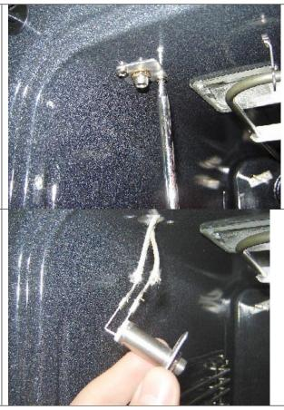
**8.3** Unscrew the nut which hold the meat probe receptacle to its mounting panel
