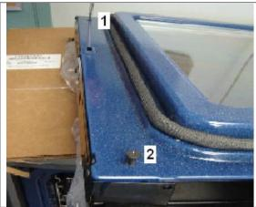
**16.3** Remove the center screw of the lower trim; the one closest from the oven door glass.
