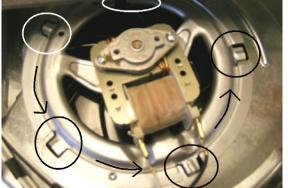
**5.5** Remove the 2 wires and the 2 screws that hold the safety thermostat.
