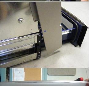
**1.7** Remove the 6 screws from the control panel as shown.
