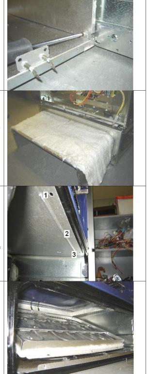
**13 15** Remove the four screws that hold the hidden bake element to its service panel.
