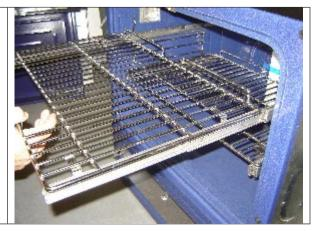
**7.3** Lift the oven rack up from both sides in order to free the glide from the ladder racks.
