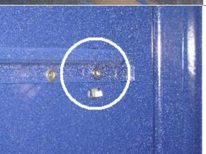
**6.10** Remove the 2 screws which hold the hinge receptacle.
