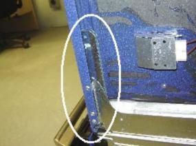
**6.12** Push the insulation back into its original emplacement making sure that it's properly tucked in behind the lower panels.
