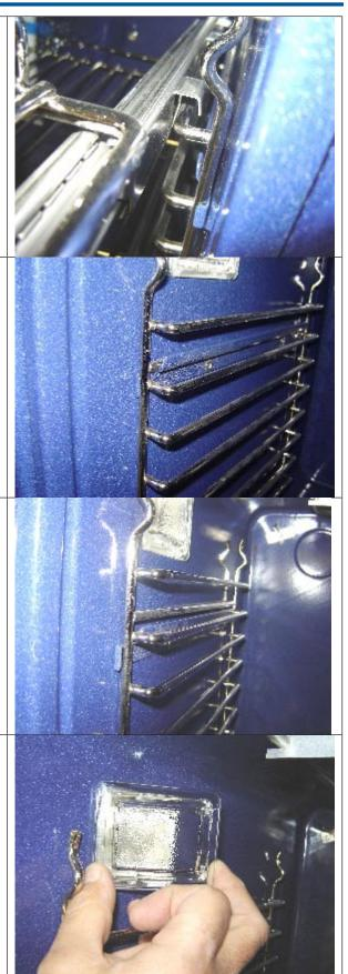
**7.6** Gently pull on the halogen lamp in order to remove it from its socket.
