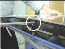
**16.4** Remove the 10 screws that hold the front decorative glass assembly; 4 at the top and 3 on each of the left and right hand side.
