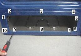
**13.3** Remove the 2 screws that hold the side of the mini oven to the frame of the unit
