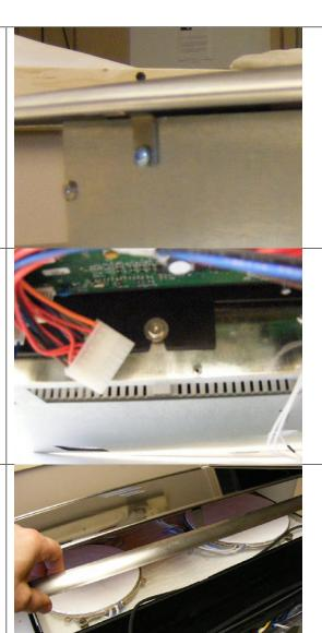
**4.5** Lift the insulation, locate service panel screw and remove it. Remove the service panel.
