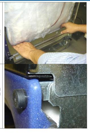
**6.13** Upon replacing the side panel, make sure that it will be inserted between the frame and the upper side panel as shown.
