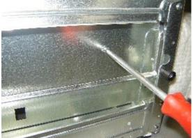
13.6 Remove the 3 screws from under the back panel of the mini oven. 13.7 Remove the wires from the mini oven sensor, mini oven light and mini oven element. **13.8** Insert these wired between the upper and lower frame as shown. 13.9 Pull the back panel off from the mini oven starting by pulling the lower portion away as shown.
