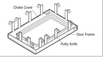
Figure 4-7. Door Disassembly
