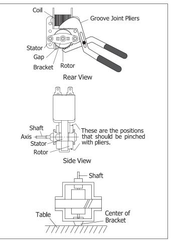
Figure 4-5. Fan Motor Components
