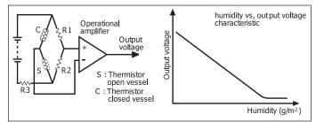
Figure 2-5. Humidity Sensor Operation
