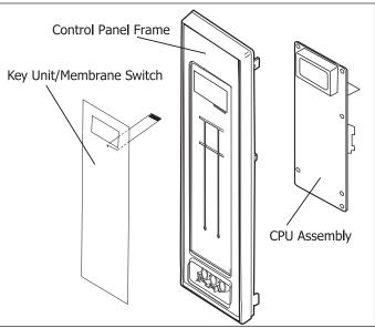
Figure 4-4. Control Panel Removal
