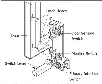
Figure 4-6. Latch Switch Adjustments
