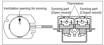
Figure 2-4. Humidity Sensor Diagram
