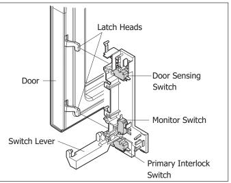
Figure 2-3. Door Open Mechanism
