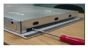
• Remove the burner box from the glass top.
