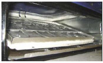
Remove the 4 screws which holds the hidden bake element to its service panel.
