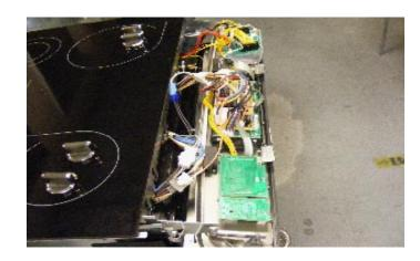
The EOC (electronic oven controller) is located in the center, as for the UIB (user interface board) it is located on the right.
