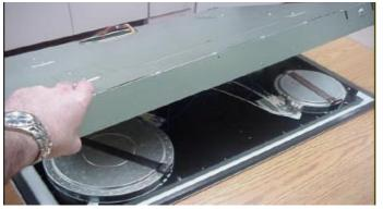
Remove the retainer bar by applying pressure to the extremity and pulling the anchorage away from the retainer bar in order to free the surface element.
