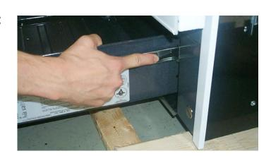
Remove the main back cover by removing the 10 screws.
