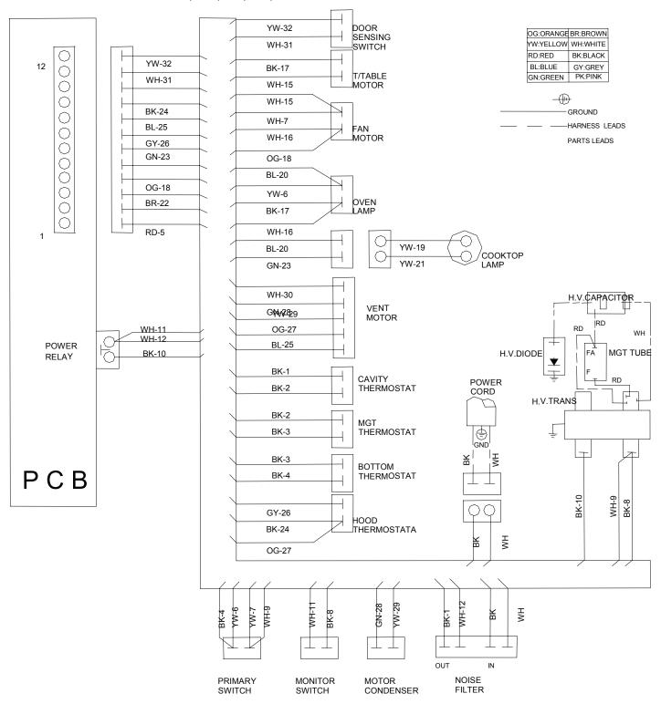
NOTE: For servicing replacement use 16GA,105 C thermoplastic covered wire except for high voltage leads or as noted on special leads.
