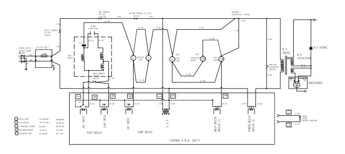
Figure O-2. Oven Schematic-Cooking Condition
