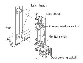
Figure D-1. Door Open Mechanism
