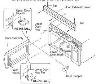
Figure C-2. Door Replacement and adjustment
