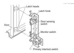
Figure C-1. Latch Switch Adjustments
