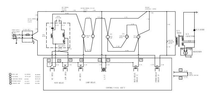
Figure O-1. Oven Schematic-Off Condition
