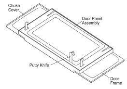
Figure C-5. Door Disassembly
