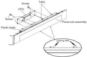
Figure C-6. Panel Angle Removal
