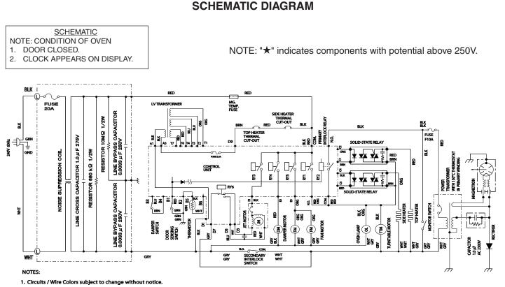
Figure O-1. Oven Schematic-OFF Condition
