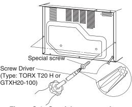
Figure C-1. Special screw postion
