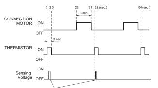
Sensing the voltage across temperature measurement circuit.
