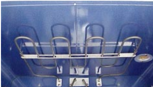
convection element and fan blade mounted to the rear wall of the oven,
