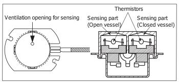
Figure 2-4. Humidity Sensor Diagram
