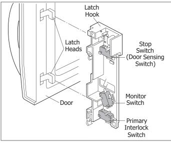
Figure 4-8. Latch Switch Adjustments
