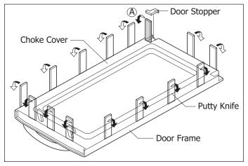
Figure 4-10. Door Disassembly
