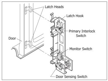
Figure 2-3. Door Open Mechanism
