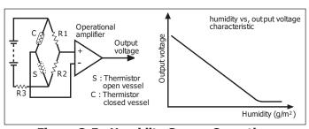
Figure 2-5. Humidity Sensor Operation
