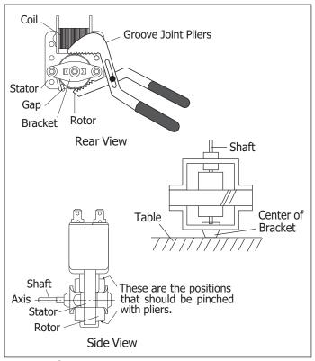
Figure 4-4. Fan Motor Components
