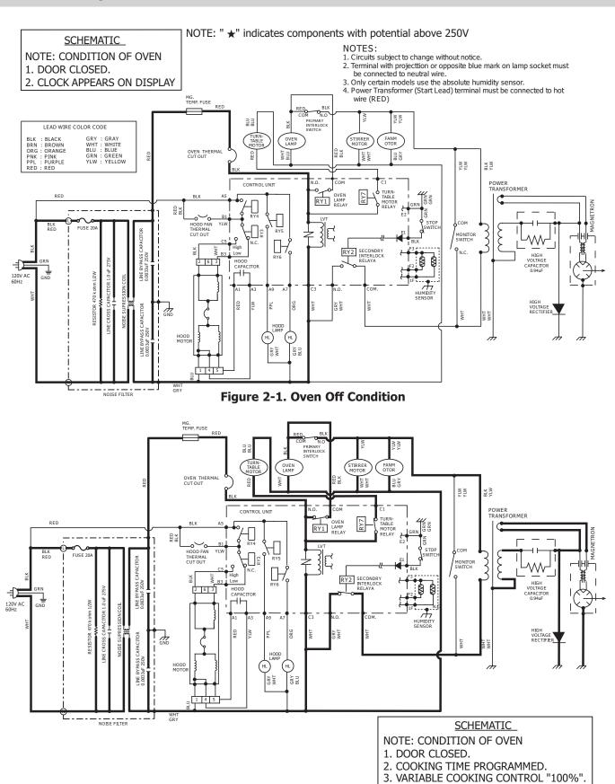
Figure 2-2. Oven ON (Cooking) Condition
