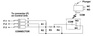
Sensor Dummy Resistor Circuit
