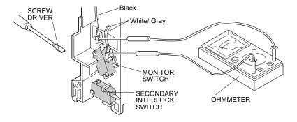
through the lower latch hole on the front plate of the oven cavity with the door opened (in this condition the plunger of the monitor switch is pushed in), the meter should indicate an open circuit. If improper operation is indicated, the switch may be defective. After testing the monitor switch, reconnect the wire lead to the monitor switch (COM) terminal and check the continuity of the monitor circuit.
