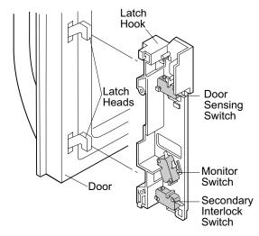
Figure D-1. Door Open Mechanism.
