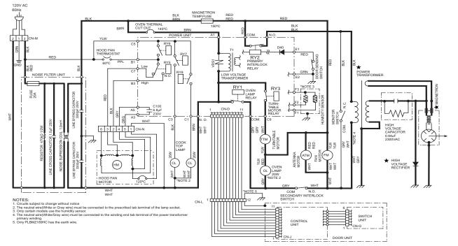
Figure O-2. Oven Schematic-Cooking Condition
