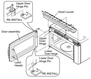
Figure C-2. Door Replacement and adjustment
