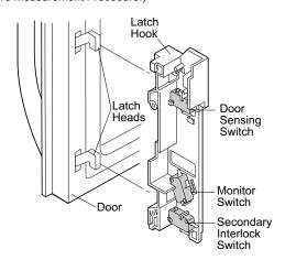
Figure C-1. Latch Switch Adjustments
