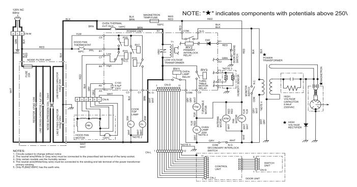
Figure O-1. Oven Schematic-Off Condition
