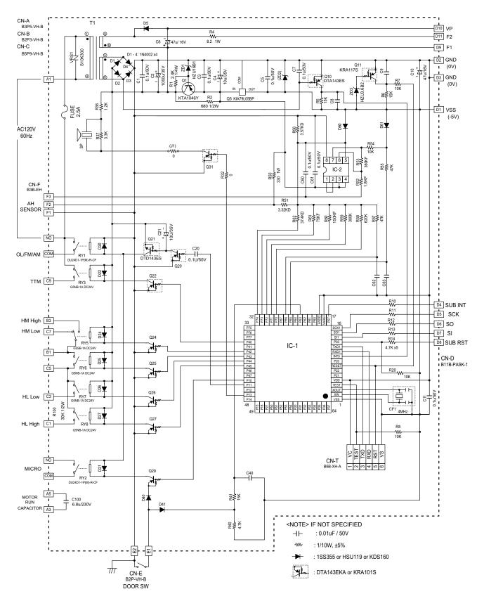
Figure S-2. Power Unit Circuit
