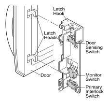
Figure D-1. Door Open Mechanism
