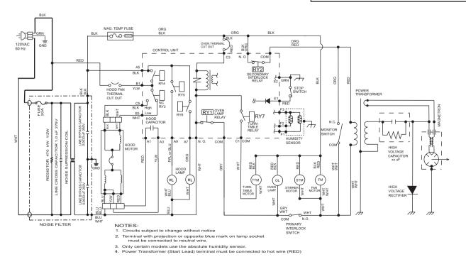
Figure O-2. Oven Schematic-Cooking Condition
