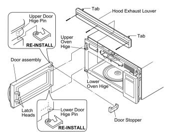
Figure C-2. Door Replacement and adjustment
