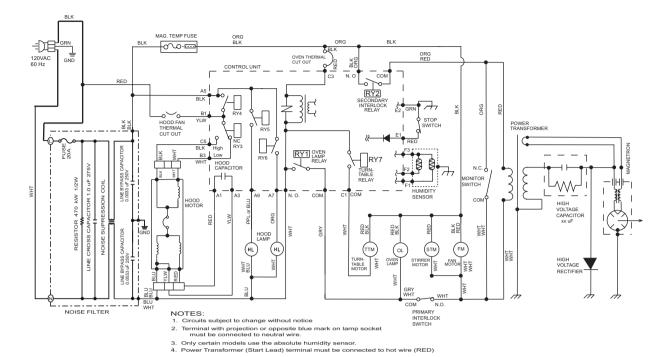
Figure O-1. Oven Schematic-Off Condition
