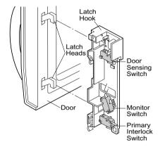
Figure C-1. Latch Switch Adjustments
