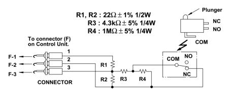
**Sensor Dummy Resistor Circuit**
