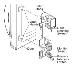
Figure D-1. Door Open Mechanism
