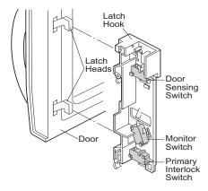
Figure C-1. Latch Switch Adjustments
