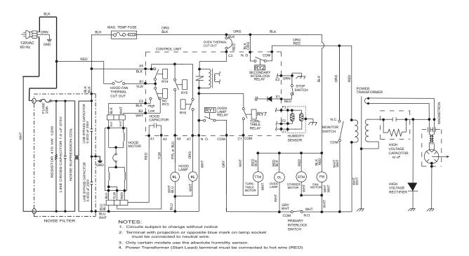
Figure O-1. Oven Schematic-Off Condition
