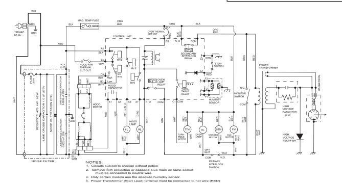
Figure O-2. Oven Schematic-Cooking Condition
