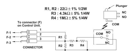
**Sensor Dummy Resistor Circuit**
