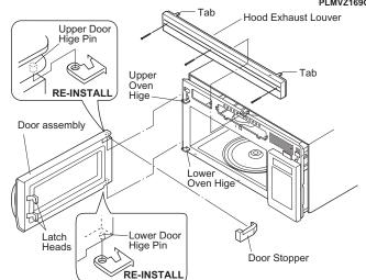
Figure C-2. Door Replacement and adjustment
