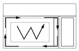
moving the probe in a clockwise direction at a rate of 1 inch/sec. If the leakage testing of the cabinet door seam is taken near a corner of the door, keep the probe perpendicular to the areas making sure that the probe end at the base of the cone does not get closer than 5cm to any metal. If it gets closer than 5cm, erroneous readings may result.
