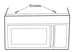
Remove 2 grille screws to remove the grill
