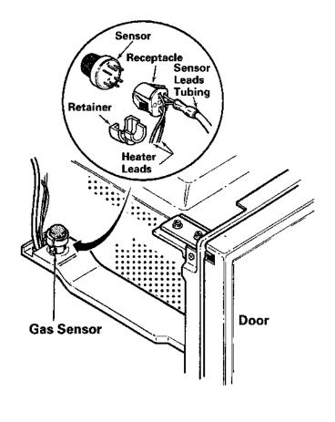
NOTE: Only heater terminals (H) can be checked with ohmmeter (30 Ohms).
