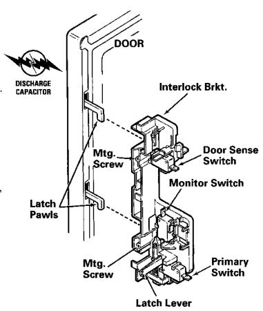
placed where the door sensing switch and primary interlock switch have activated with the door closed.
