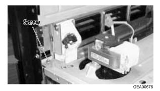
3. Remove 2 screws via the damper screw access holes.
