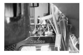
Remove 2 screws holding the thermistor in place. Access the screws through the access ports.
