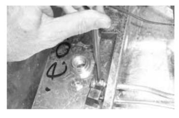
3. Remove the 5/8-in. nut on the jet holder and remove the jet holder.
