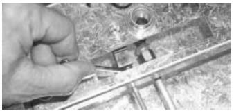
3. Remove the 5/8-in. nut on the jet holder and remove the jet holder.
