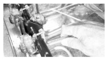
6. Remove two 5/16-in. nuts and the valve.
