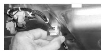
8. Push the spark electrode wires through the holes in the maintop.
