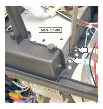
**Note:** The 2 front screws are recessed from the top of the metal shield. Access holes are provided. A magnetic screwdriver is necessary to capture these screws.
