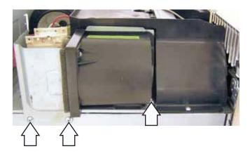
7. Remove the 4 Phillips-head screws and the duct from the Upper Cooling Motor.
