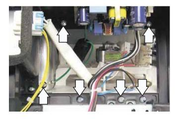
15. Push the top of the cooling fan cover toward the rear of the oven, then carefully lift the baseplate from the oven.
