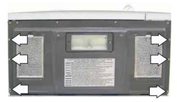
3. Remove 7 Phillips-head screws from the back of the oven.
