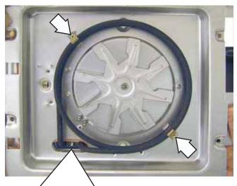
The convection heater element is held in place by 3 Phillips-head screws. (Two screws on the front, and 1 screw on the end.)
