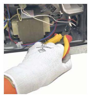
**Note:** The capacitor has an internal discharge resistor that automatically discharges the capacitor when the oven turns OFF. Under normal operation, capacitor should fully discharge within 30 seconds.
