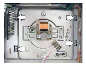
19. Position the damper toward the front of the oven, then lift the bottom of the Convection Heater Assembly out from the oven.
