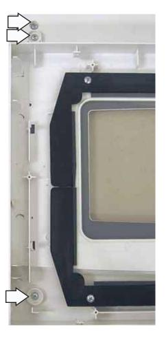
7. Remove the 6 Phillips-head screws that attach the top and bottom glass retainers to the door frame.
