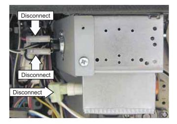
**Note:** In the following step, an overlapping metal shield may limit access to the 2 rear screws that attach the Magnetron to the oven. It may be necessary to pry back the shield while removing the 2 screws.
