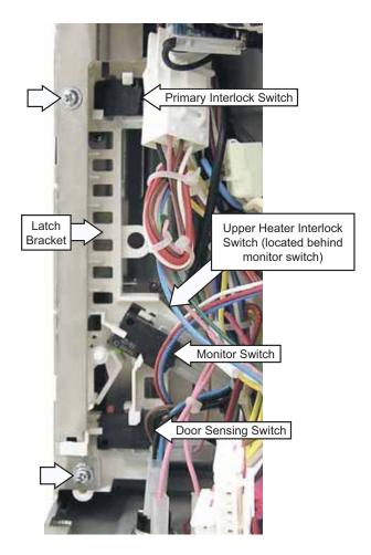
4. Using a small flat blade screwdriver, release the tabs and remove the door switch from the latch bracket.
