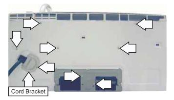
7. Slide the Outer Cover back about 1 inch toward the rear of the oven, then lift the cover from the oven.
