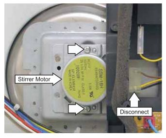
**Caution:** When installing the Stirrer Motor, misalignment of the stirrer blade hub can damage the stirrer cover. Before installing the Stirrer Motor, use a screwdriver inserted into the stirrer blade hub to pre-align the square drive of the stirrer blade to allow engagement of the motor shaft.
