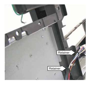
17. Push wiring thru the entry hole, then remove the Air Tunnel Inlet.
