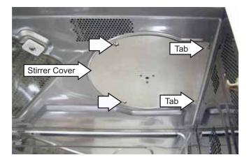
4. Lift the stirrer blade off the pin embedded in the cover.
