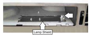
4. Lift the right side of the shield and remove it from the opening.
