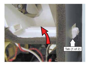
6. Push the top of the fan cover toward the rear of the oven, then carefully remove it from the oven.
