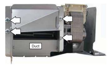
8. Remove the Phillips-head screw that attaches the bottom plate and side plate to the Upper Cooling Motor.
