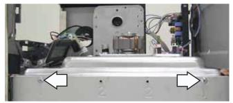
18. Remove the four 7-mm hex nuts that attach the Convection Heater Assembly to the oven.
