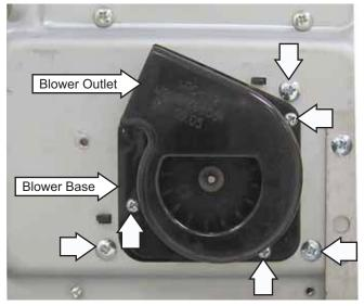
7. Move the Lower Cooling Motor toward the right and carefully maneuver the Lower Cooling Motor out from the oven.
