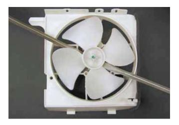
8. Remove the 2 Phillips-head screws that attach the fan motor to the fan cover.
