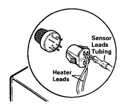
NOTE: Only heater terminals (H) can be checked with ohmmeter (30 Ohms).
