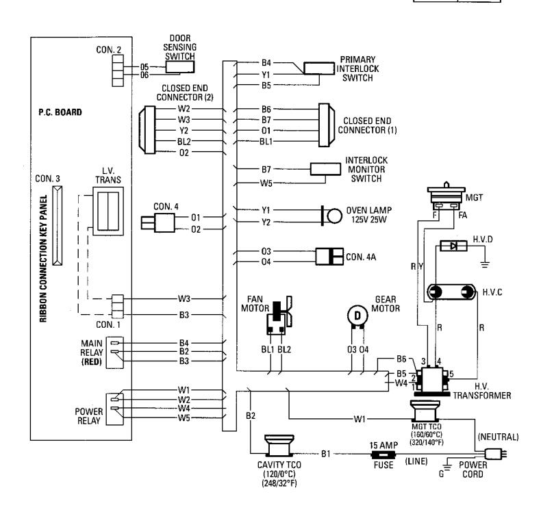
NOTE 3: All leads that enter common lead path (\_\_\_\_\_\_ must be traced to their terminations. Con. 4 and 4A are connected together.
