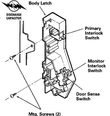
placed where the door sensing switch and primary interlock switch have activated with the door closed.
