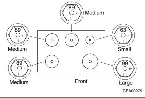
burner chimney as shown by number on the above chart:
