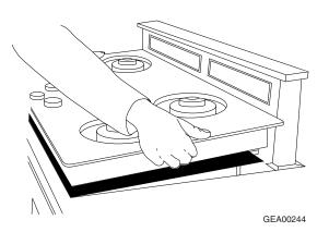
2. To ensure a good fit, position cooktop over cutout opening and carefully lower into place. Check edges all the way around to be sure all cutout edges are concealed and there are no gaps.
