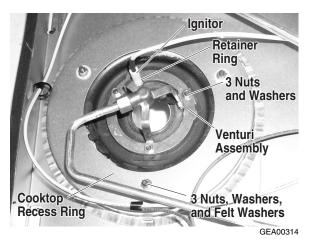
**WARNING:** Disconnect electrical power to the cooktop and turn OFF gas at the main valve before performing any removal procedures.
