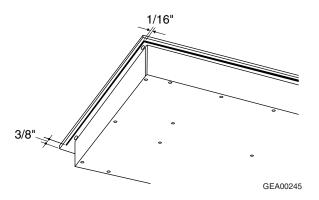
4. Cut a 3/16-in. gasket strip in half. Peel off backing and apply to underside of glass cooktop edge, on each side at least 3/8 in. from the back and as close to the edge as possible without protruding. 5. Apply the other gasket strip to underside of glass at front of cooktop.
