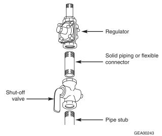
**Note:** When using test pressures greater than 1/2 psig to pressure-test the gas supply system of a residence, disconnect cooktop and individual shut-off valve from gas supply piping. When using test pressures of 1/2 psig or less to test the gas supply system, simply isolate cooktop from gas supply system by closing individual shut-off valve.
