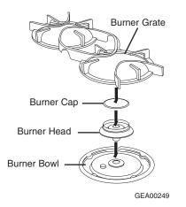
Place burner heads and caps on burners. Make sure that heads and caps are placed on correct size burner. There are 1 small, 2 (or 3) medium, and 1 large head and cap.
