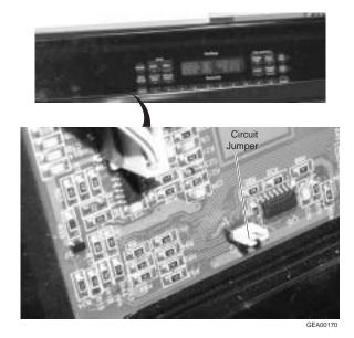
**NOTE:** On the circuit board behind the control panel is a circuit jumper that may fall off during disassembly. When reconnecting the jumper, be sure to position it on the left and center pins. *Incorrect assembly of the circuit jumper will result in ECP failure.*
