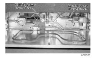
**NOTE:** Electrical warming components are accessible when the warming drawer is removed.
