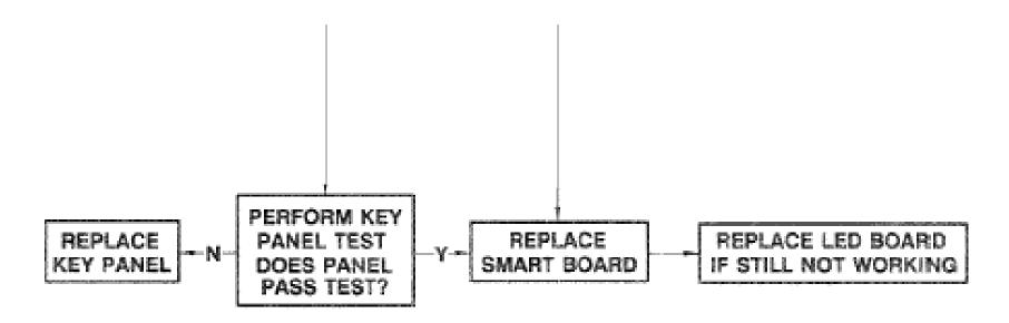
\*NOTE: WHEN CONNECTORS ON SMART BOARD & LED BOARD ARE SWITCHED, CONTROL WILL OPERATE OPPOSITE DIAGONAL UNIT. (EXAMPLE) RIGHT FRONT KEY PADS WILL CONTROL LEFT REAR UNIT.
