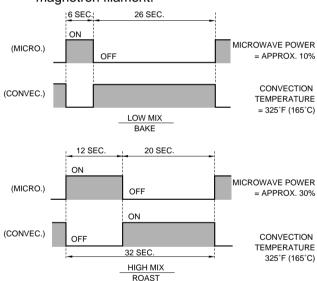
Note: During alternate Microwave/Convection operation, the convection heater is energized only if the cavity temperature drops below the set temperature.
