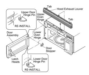
Figure C-2. Door Replacement and adjustment
