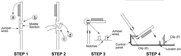
POSITIVE LOCK® CONNECTOR (NO-CASE TYPE) REMOVAL
