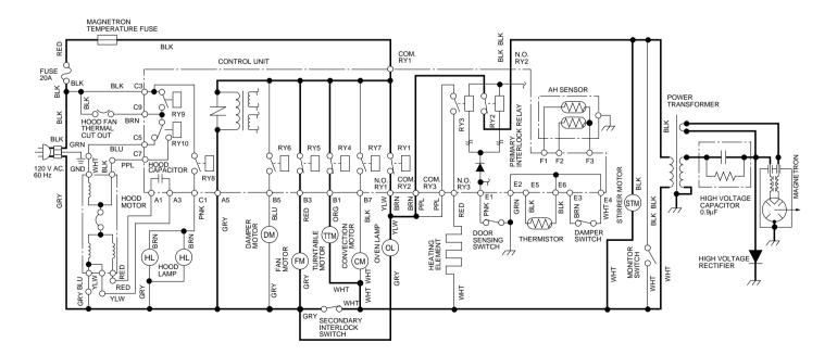
Figure O-2. Oven Schematic - Microwave Cooking Condition
