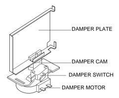
Figure D-2. Damper Mechanism
