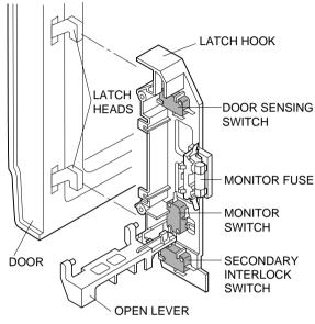
Figure C-1. Latch Switch Adjustments
