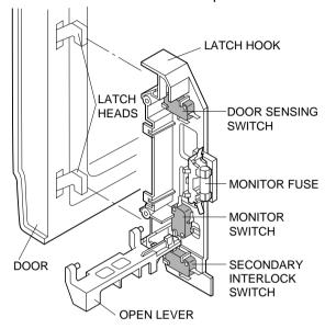
Figure D-1. Door Open Mechanism
