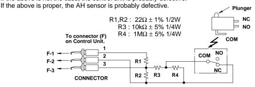
**Sensor Dummy Resistor Circuit**
