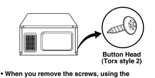
When you remove the screws, using the tamper-resistant Torx driver have a pin-in-head.
