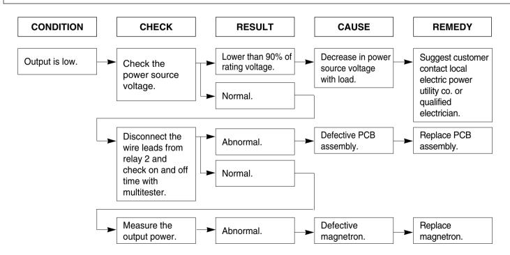
**NOTE:** Simple test of power output-conducted by heating one liter water for one min. if available. Minimum 8.5°C temperature rise is normal condition.
