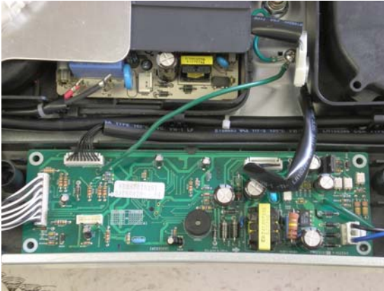
CN 1 and CN 2 are shown reversed, as described in Step 2.
