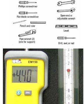
For the most part, ordinary hand tools are sufficient for installing the range. It will be necessary to check the incoming gas pressure and to regulate it if it is out of specification.
