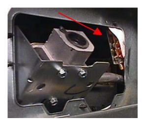
LP orifice spuds are located at the back of the warming drawer compartment. The spuds are in a metal bracket next to the pressure regulator and are attached to the back wall of the compartment by a <sup>1</sup>/<sub>4</sub>" hex head screw.
