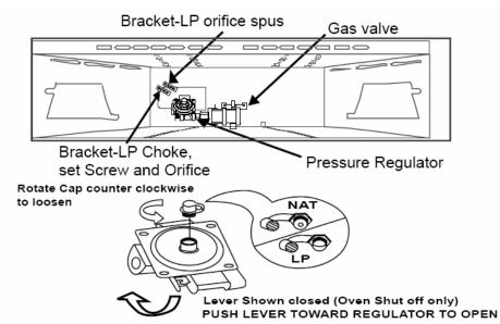
Remove the grates, burner caps, and burner heads. Then remove the brass orifice (spud) in the chimney of each burner using a  ${}^{9}/_{32}$ " (7 mm) wrench or nut driver.
