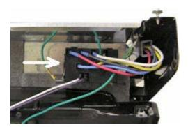
The spark module is in the back guard and held in place by two plastic tabs, one on each side. Put the control panel into service position, and press either tab to remove the module.
