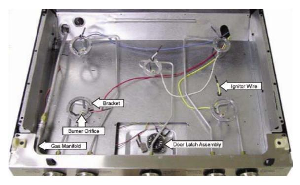
Cooktop removed, with heat shield and latch assembly cover removed
