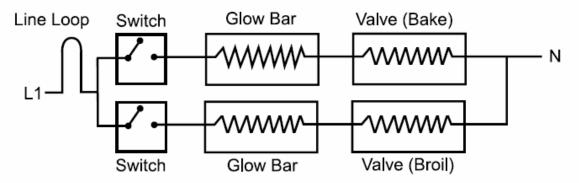
As shown in the schematic, the valve is in series with the ignitor (glow bar). When 120  $V_{AC}$  is applied, the ignitor requires a minimum of 116, leaving only about 4 volts to operate the valve. The ignitor will remain energized at all times the burner is operating.
