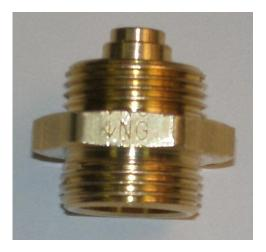
The hex nut is marked with NG for natural gas and LP for propane. There is an arrow showing which way to install the nut.
