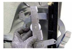
Position the top of the hinge body into the notch in the hinge arm (see photo) and rotate the hinge body clockwise to remove.
