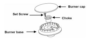
For the extra large burner (right front), the choke and self threading screw will be needed. Insert the choke into the burner base, then insert the set screw into the burner base and tighten securely. Make sure the screw head is against the shoulder (within the choke notch), so it does not have any rotational movement.
