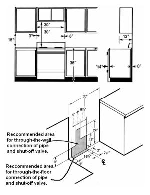
This drawing shows the minimum clearances for the gas range. The 30" requirement between stovetop and cabinet bottom allows sufficient space to the installation of a standard overthe-range microwave oven.
