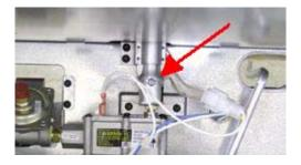
To correct a BAKE flame problem, remove the warming drawer, loosen the air shutter, and adjust the opening to  $^{11}/_{16}$ ". Run the flame test. If the flames are yellow, open the shutter an additional  $^{1}/_{32}$ ". If they lift off or flutter, close it by  $^{1}/_{32}$ ". Repeat the flame test until the flame is acceptable.
