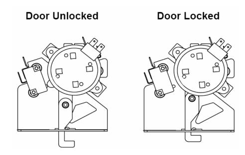
As the cam revolves about  $\frac{1}{2}$  revolution (approximately 12 seconds), it has moved the lock hook into a corresponding slot in the oven door which secures the door.
