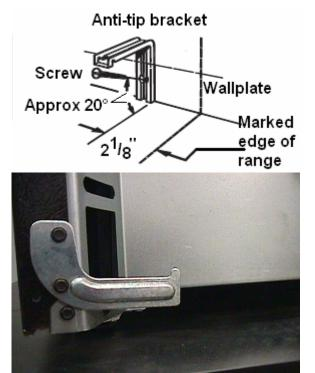
Be sure to install the anti-tip bracket. This prevents tipping the range in the event someone stands on the door or otherwise puts the range off balance. Use the installation template to locate the wall bracket; then, attach the bracket to the wall with a large wood screw.
