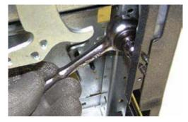
Remove the two ¼" hex head screws that attach the hinge to the frame.
