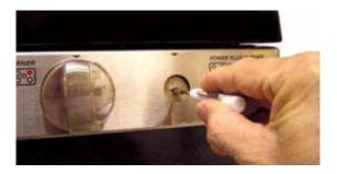
Remove the surface control knob and locate the adjustment screw in the center of the control valve shaft. A thin flat-blade screwdriver, approximately  ${}^{3}\!/_{32}$ " across, is needed to access the screw. Turn the adjustment screw until the flame reaches the desired size.
