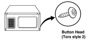
When you remove the screws, use the tamper-resistant Torx driver having a pin-in-head.
