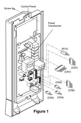
(4) Remove 3 screws securing the circuit board.
