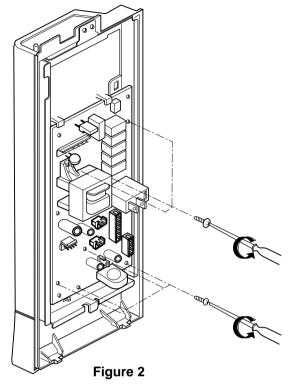
(5) Remove the circuit board from the control bracket carefully.
