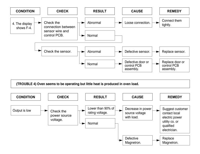
**NOTE :** Simple test of power output-conducted by heating one liter water for one min. if available. Minimum 8.5°C temperature rise is normal condition.
