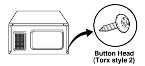
When you remove the screws, using the tamper-resistant Torx driver have a pin-in-head.
