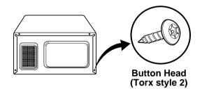
When you remove the screws, use the tamper-resistant Torx driver having a pin-in-head.
