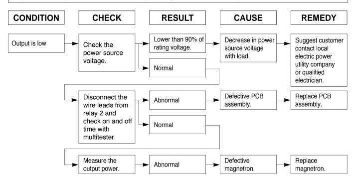
NOTE: Simple test of power output-conducted by heating one liter water for one min. if available.
