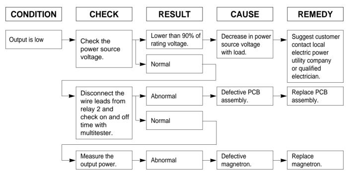
NOTE: Simple test of power output-conducted by heating one liter water for one min. if available.
