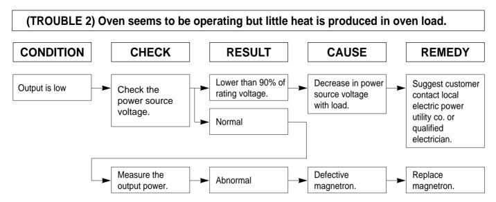
NOTE : Simple test of power output-conducted by heating one liter water for one min. if available. Minimum 8.5°C temperature rise is normal condition.
