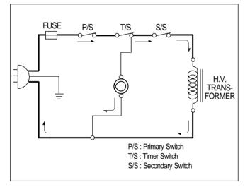
• 3.2 volts AC is generated from the filament winding of the high voltage transformer. This 3.2 volts is applied to the magnetron to heat the magnetron filament through two noise-preventing choke coils.
