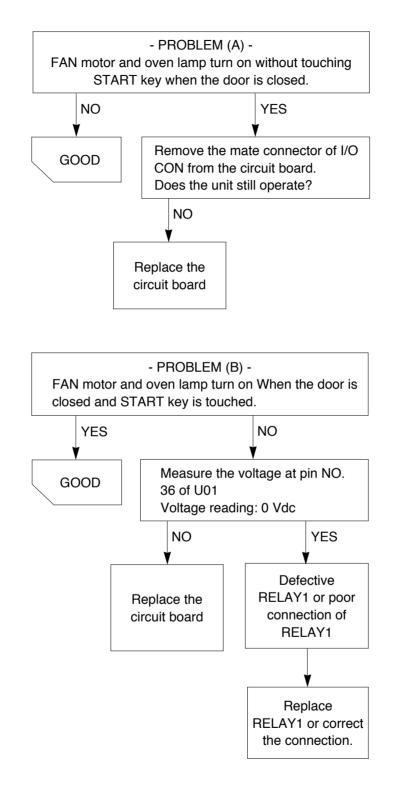
(3) CHECKOUT PROCEDURES FOR CIRCUIT BOARD
