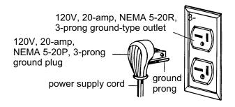
If a mating outlet is not available, it is the personal responsibility and obligation of the customer to have a properly grounded, NEMA 5-20R, 3-prong outlet installed by a qualified electrician.
