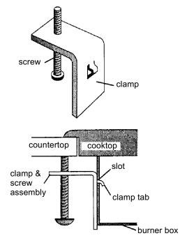
4. Secure the cooktop to the countertop by hand-tightening each screw, then use a screwdriver to tighten each screw by 1 to 1-1/2 more turns. Do not overtighten.
