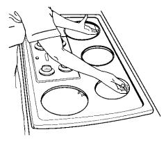
3. Rotate the support rod against the front of the burner box.
