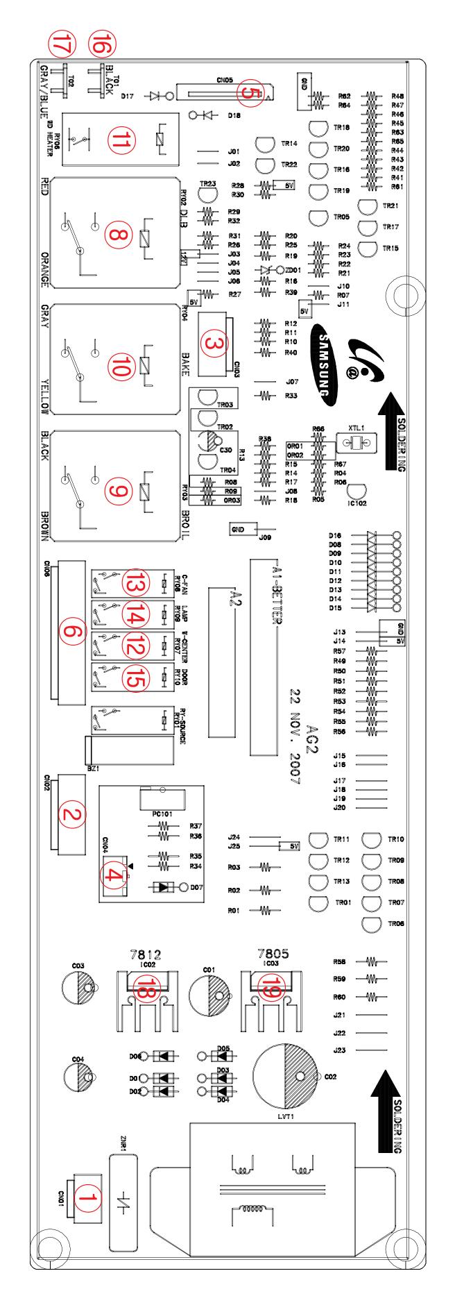
6. PCB Diagrams **6-2 PCB Diagrams** (This Document can not be used without Samsung's authorization) RY02 1) DLB 2) DLB CN05 Key Pad Connector T02 1) W/Drawer Relay T02 1) W/Drawer Relay Relay Relay Terminal1Terminal2 RY04
