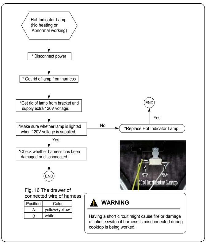
(\* Warning : Having a short circuit of harness color to be turned "Yellow+white" might cause fire or damage of infinite switch.)
